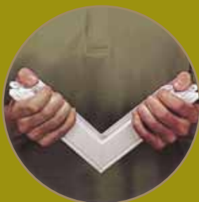
Pinch fusion welding
